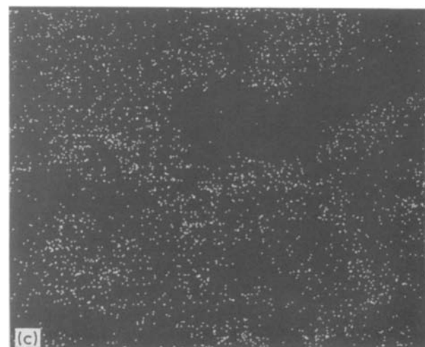
Figure 9 SEM and EDX analyses of \text{ZnAl}_2\text{O}_4 formation in a specimen of agglomerate of fine \text{Al}_2\text{O}_3 , ZnO and LiF fired at 800^\circ\text{C} for 20 h. (a) SE image, (b) X-ray image of zinc, (c) X-ray image of aluminium.
